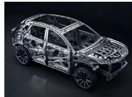
SAFE BODY STRUCTURE 85% HIGH-STRENGTH STEEL
