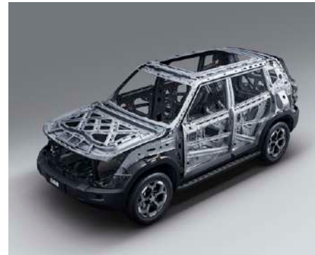
SAFE BODY STRUCTURE 85% HIGH-STRENGTH STEEL
