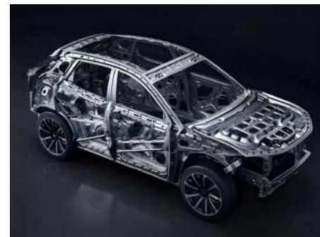
SAFE BODY STRUCTURE 85% HIGH-STRENGTH STEEL
